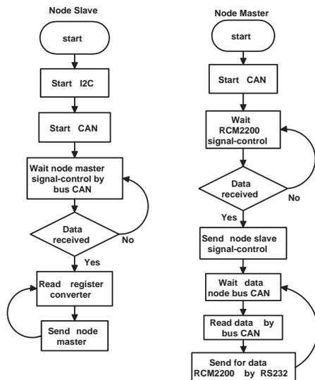
Fig. 5. Firmware of the microcontrollers nodes.
