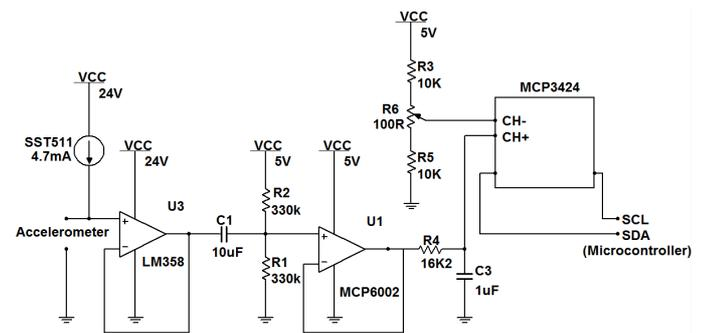
Fig. 3. Conditioning circuit for an accelerometer.
