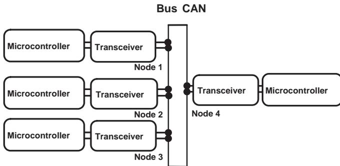
Fig. 4. Diagram of the CAN bus.
