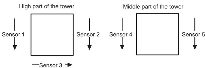
Fig. 2. Positioning of the accelerometers in the tower
