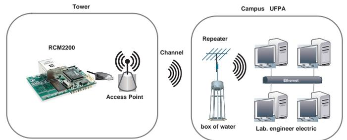
Fig. 6. Diagram of the data transmission system.
