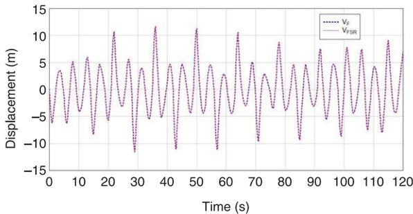
Fig. 5. Vertical displacement time histories for a section located at the center of the cable comparing the case which considers only bending and geometrical stiffness,  $V_F$ , with the most general case,  $V_{FSR}$ .
