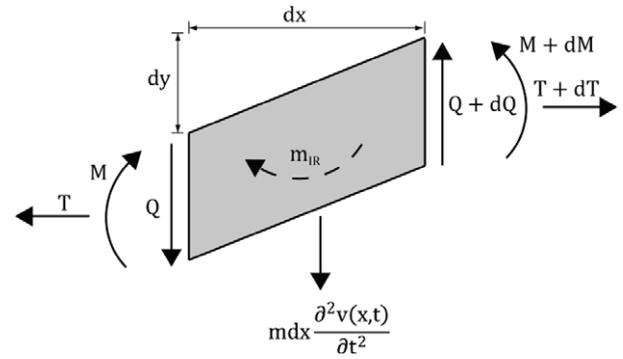
Fig. 1. Infinitesimal element considering rotational inertia.
