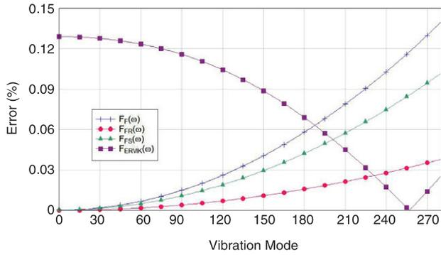
Fig. 3. Error corresponding to functions  $F_F(\omega)$ ,  $F_{FR}(\omega)$ ,  $F_{FS}(\omega)$ ,  $F_{ERVIK}(\omega)$  with respect to function  $F_{FSR}(\omega)$ .
