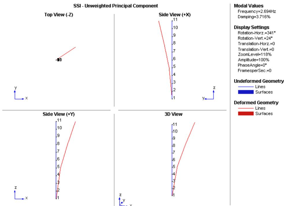
**Figure 3.** Model 2 – 1st mode, freq = 2,694 Hz – ARTEMIS
