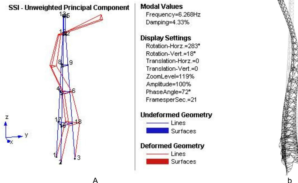
**Figure 2.** Modal shape for Model 3. a: Mode 6 of ARTeMIS Extractor, b: Mode 10 of SAP2000.
