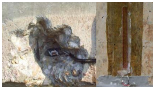
Fig. 7 Extensometria no concreto [1]
